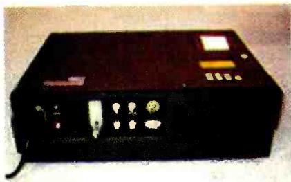
THIS PORTABLE, REAL-TIME ASBESTOS-MEASURING DEVICE was developed by Toyo University's Department of Engineering and the Escom Corporation. It could also be adapted to measure other types of airborne particles.
